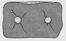
Lint will blow into the heat exchanger through cracks and tears. This will cause a permanent obstruction in the heat exchanger. White residues or residues of other colors
