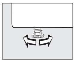
The screw feet can be adjusted to compensate for unevenness in the floor.
