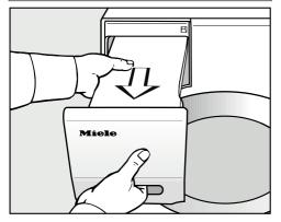
Remove the condensed water container.
