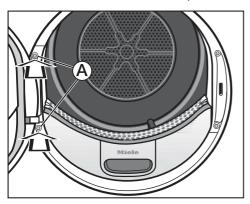
■ Screw the door securely to the dryer at the base of door hinge (A).
