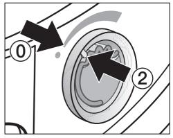
■ Turn the outer ring counterclockwise until marker ② is in position ③.
