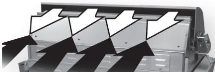
Be sure wind doesn't blow into the hood gap.
