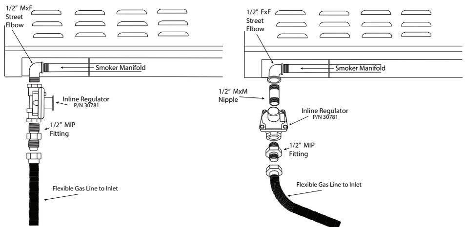
Never run flex hose behind the firebox, run the hose at an angle, straight down, or out of the back.
