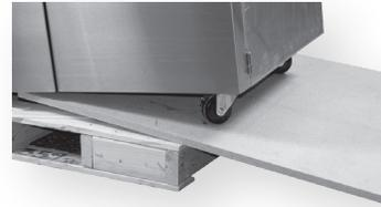
lifting one end of the smoker high enough to place a ramp under the wheel and then lift the other end while rolling the smoker off of the pallet.
