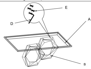
step 1:Turn over,use screw (E) connect the stainless steel base (B) with the stainless steel base (A) by Allen key (D).
