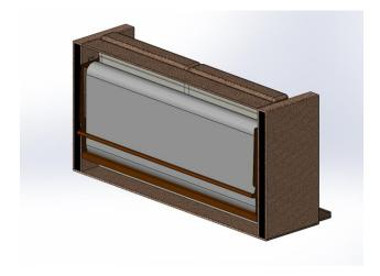
Step 2: Press sleeper unit inwards to expose the connector bracket.
