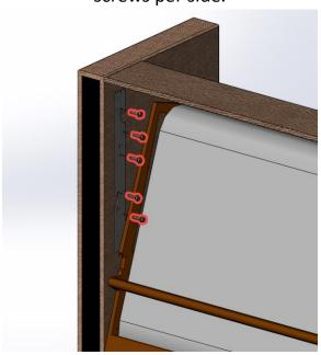
Step 4: Pull sleeper mech out from bottom.
