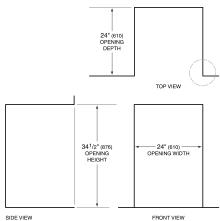
NOTE:  $3^{1/2^{\prime\prime}}$  (89) finished returns will be visible and should be finished to match cabinetry.
