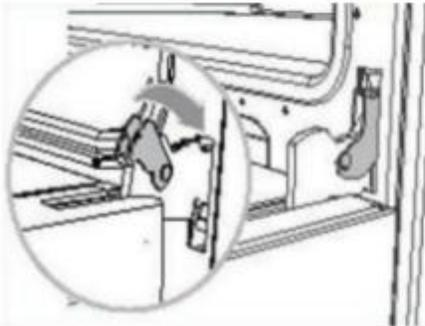
4. Fully close the levers on the left and right hinges, as shown, then close the door.
