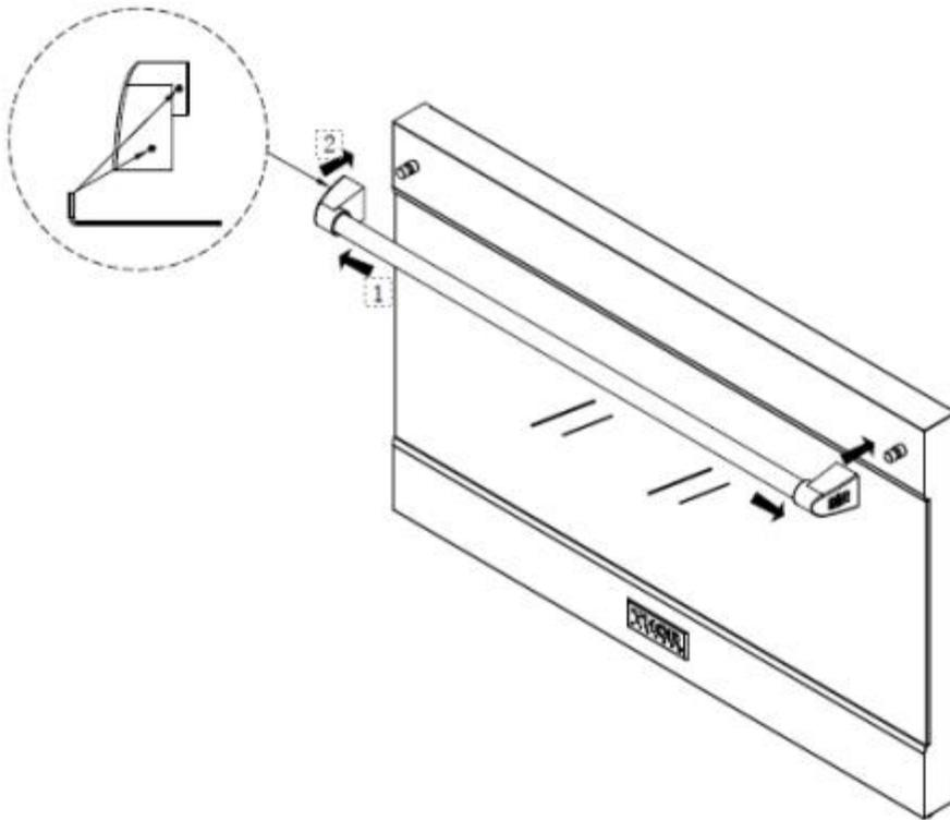
3.2 Insert the handle tube into the left and right handle seat.
