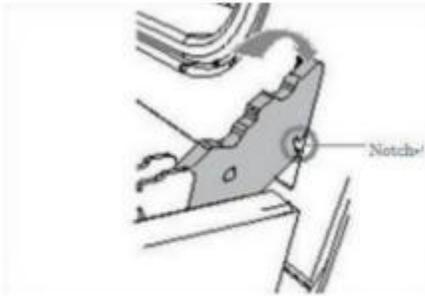
2. Insert the hinge tongues into the slots making sure that notches on both sides drop into place as shown.
