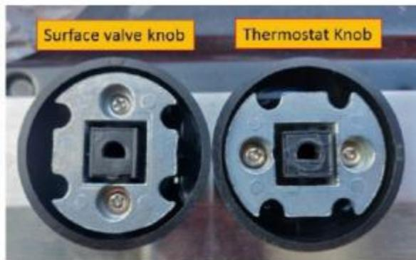
{Incorrect knob caused broken thermostat shaft}
