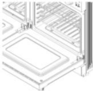
4. Take apart and remove the hinge, close it gently about half way through the door, and place it on the protective surface.
