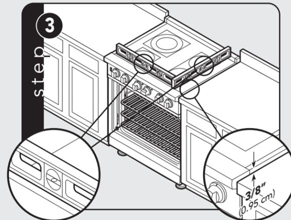
Check that unit is level side to side and front to back. The side trim must be  $\frac{3}{8}$ " (0.95 cm) above countertop. If unit is not level repeat steps 5-7 of "Leveling/Adjustments/Alignment" section.
