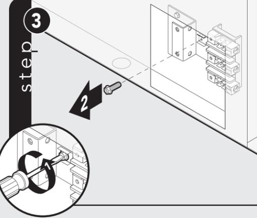
Remove grounding screw. Cut-off and discard ground strap.
