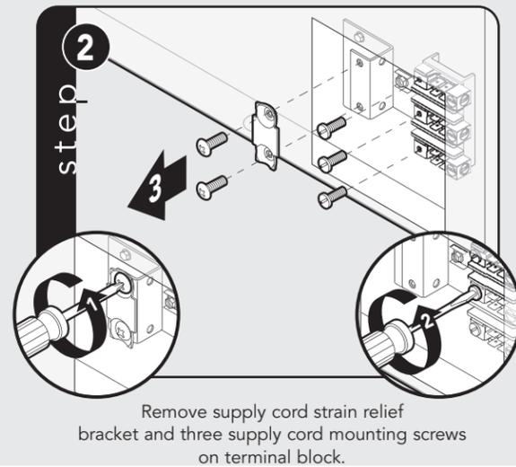
Remove supply cord strain relief bracket and three supply cord mounting screws on terminal block.
