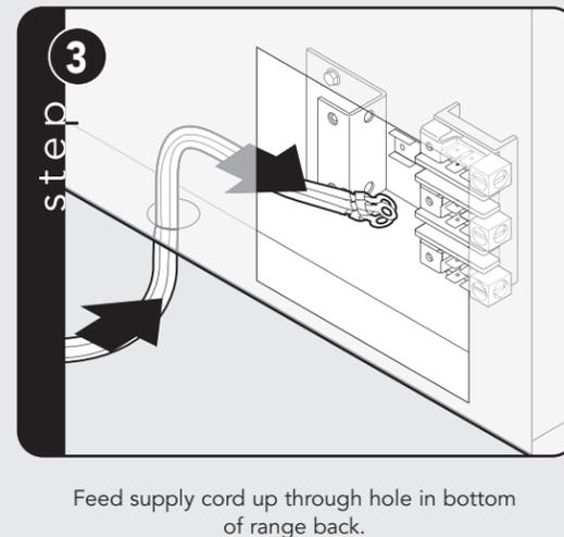
Feed supply cord up through hole in bottom of range back.
