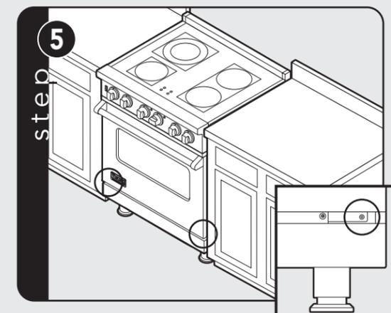
If the door needs to be adjusted, loosen hinge trim screws (see step 2). Adjust the screws located between the door and kickplate using a  $\frac{5}{32}$ " hex head allen wrench. After adjustment, tighten hinge trim screws.
