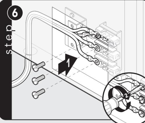
Attach line #1 (black) and line #2 (red) leads to outside terminal. Attach neutral wire (white) to center terminal on terminal block.
