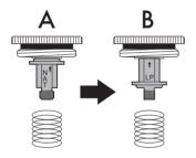
4. Screw in the regulator stem and cap into its place.
