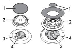
Make sure that the holes of the flamespreader crowns are aligned with the thermocouples (3) and igniters (4).
