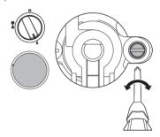
Refit the knob and verify the correct ignition and burner flame stability (when turning the knob rapidly from the maximum to the minimum position the flame must not go out). Repeat this operation on the remaining gas taps on the cooktop.
