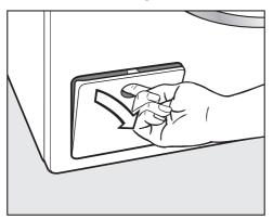
■ Open the drain pump flap.
