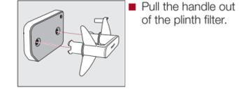
■ Pull the handle out of the plinth filter.
