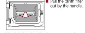
The right-hand guide pin comes out when the plinth filter is removed. The guide pin prevents the access panel from closing without the plinth filter.
