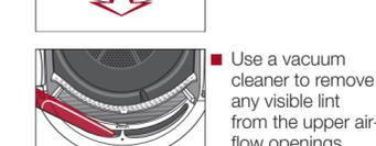
■ Use a vacuum cleaner to remove any visible lint from the upper air-flow openings.
