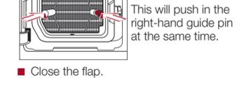
■ Push the plinth filter in completely. This will push in the right-hand guide pin at the same time.
