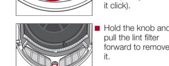
■ Hold the knob and pull the lint filter forward to remove it.
