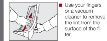
■ Use your fingers or a vacuum cleaner to remove the lint from the surface of the filter.
