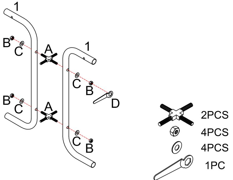
**STEP 2** Attach the two remaining Support Legs (1) to the "+" bolts (A) using 4 Washers (C) and 4 Nuts (B). Do not tighten until after you have completed the entire assembly process.
