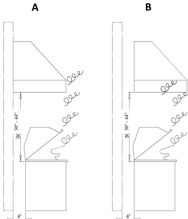
a. Install the hood at least 30", but no more than 44" above the cooking surface. If the hood is installed more than 44" above the cooking surface, its' smoke capture ability declines rapidly. See Drawing A.
