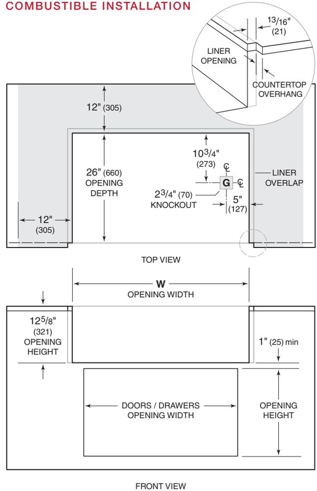
NOTE: Shaded area above countertop indicates minimum clearance to combustible surfaces, combustible materials cannot be located within this area.
