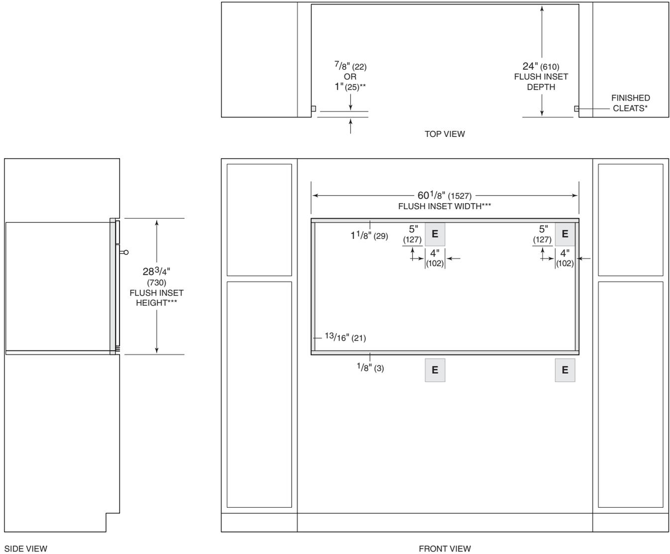
\*1" (25) minimum depth. Shaded areas will be visible and should be finished to match cabinetry.
