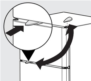
17. Tighten the top hinge screws and check door gasket for open seal condition (gap between gasket and cabinet flange).
