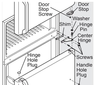
7. Remove two screws on bottom hinge with 3/8" socket wrench.
