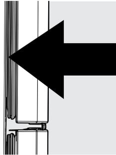
Gasket should seal against the cabinet all the way around including top and bottom
