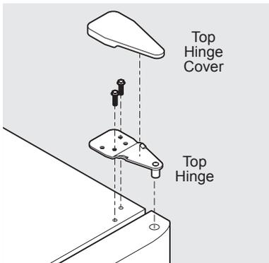
3. Unscrew center hinge pin using adjustable wrench and save for reassembly. Ensure plastic washer stays on hinge pin.
