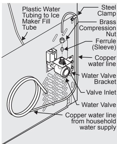
(Include enough tubing in loop to allow moving refrigerator out for cleaning.)
