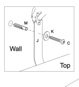
With drilling machine make one hole in the wall, Insert part (M) in the hole.
