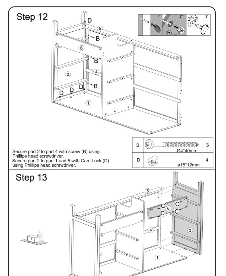
Join parts 3 and 6 to parts 1,4 and 5, secure part 6 with screw (C) using
