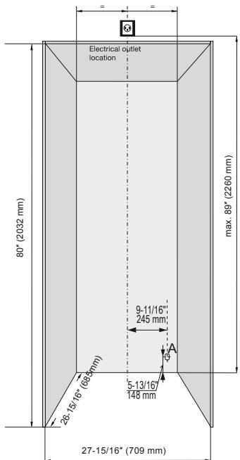
The appliance can be used freestanding or semi built-in. If semi built-in, consider the minimum cabinet opening dimensions specified on this image. For ventilation requirements, please follow instructions on section Ventilation Requirements in the Freestandig Design Guide.
