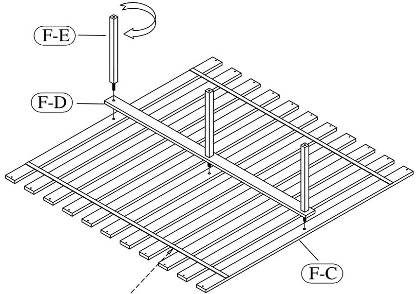
Attention : The bed slat straps should be located on the bottom side when properly installed.
