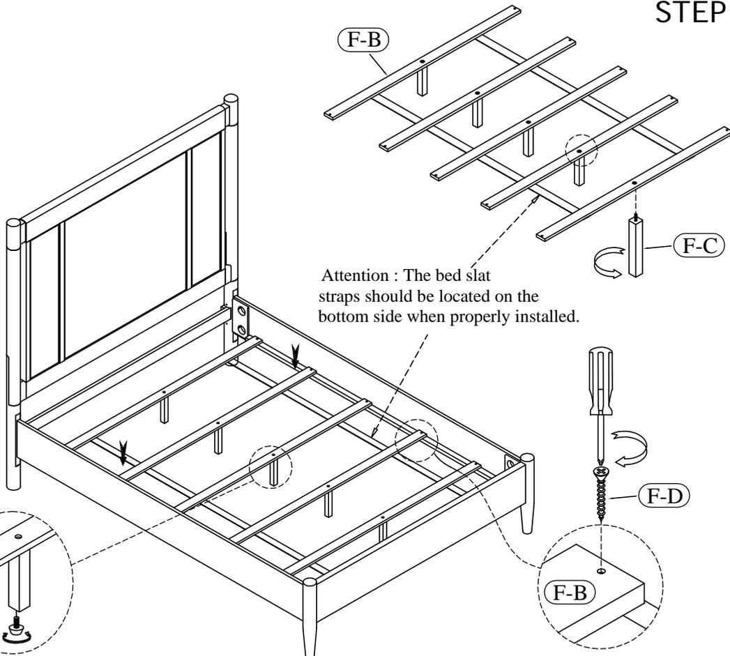
Attention: The bed slat straps should be located on the bottom side when properly installed.
