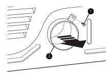
2 Press the adapter duct 3 onto the blower housing and secure it to the base of the dryer as shown.
