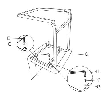
Assemble the chair seat with the chair leg but do not fully tighten the bolt(E&F).
