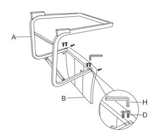
Firstly, fix the backrest with the chair leg but do not fully tighten the bolt(D).
