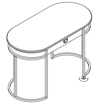
Wire management hole on back of desk: pull the disk out, run wires, and snap disk back in place.
