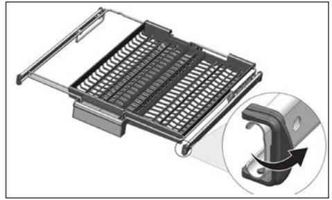
When the central tray is in the lower position, you can load long/high items such as coffee cups, ladles, etc. on the tray. When the side trays lean on two side walls, the handle can be pulled to allow the central tray to rise and the system to be locked.
