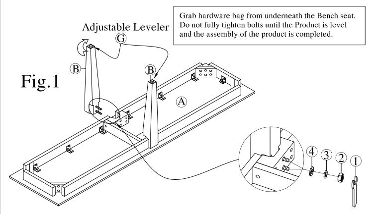
Step 1: Lay the Bench Seat (A) upside down on a flat soft surface. Insert Bench Center Leg (B) into Bench Seat (A), using the provided hardware as shown on Fig. 1. Do Not Fully Tighten Bolts Yet
