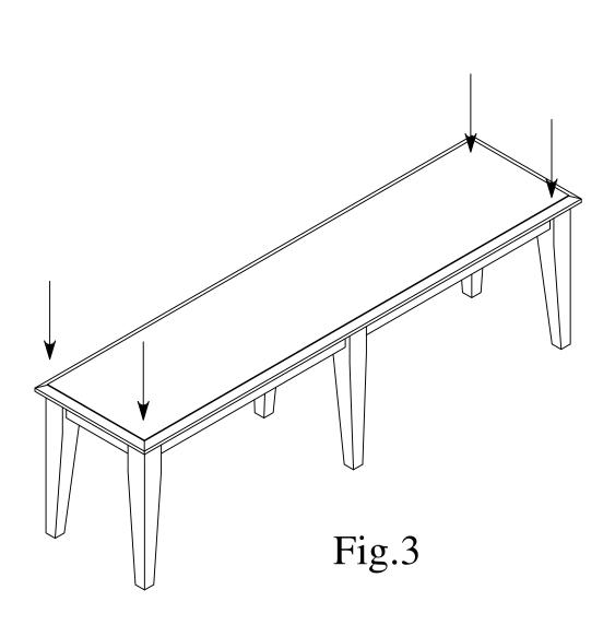
Step 3: Place the loosely assembled Bench on a hard flat surface and apply gentle downward pressure on the seat. As shown on Fig.3. Once the Bench is balanced and leveled, fully tighten all bolts.
