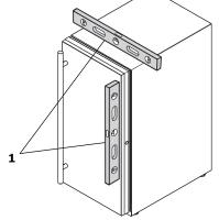
2. If the unit is not level, adjust the legs on the corners of the unit as necessary.
