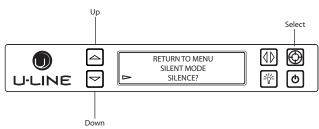
Users can halt ice production for 3 hours with an option called "Silent Mode" in the Customer Menu. Silent Mode will begin once the current ice making cycle is complete. After 3 hours in Silent Mode, normal ice production will continue.
