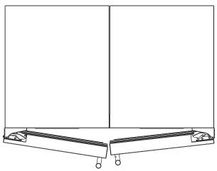
However, to ensure unobstructed door swing (opening both doors at the same time), 1/4" (6.4 mm) of space needs to be maintained between the units.
