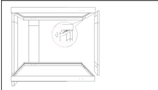
3. Repeating Step 2, screw the 2nd, 3rd, and 4th table legs onto the table top and shelf frames.
