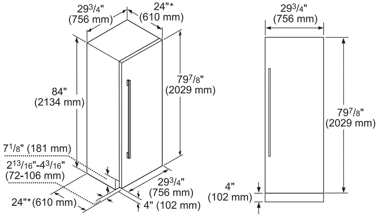
\*Excludes thickness of door panel. If standard panel with 3/4" thickness is mounted, total depth is 24 3/4".
