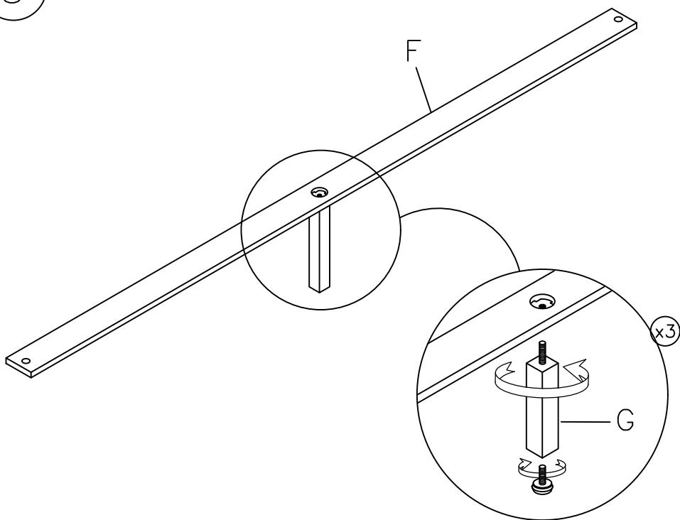
Turn Adjustable Leveler on the bottom of the Cross-Slat Support Leg leaving 6mm space between leveler and the floor.
