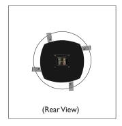
After the speaker has been inserted, secure the screws. The process of securing the screws will rotate the holding tabs to clamp onto the wall/ceiling material.
