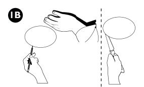
For existing installations, mark a cut-out circle/square on the ceiling/ wall. (Reference the sizing chart to find the correct dimension for your speaker.) Then cut along your traced line to cut a hole in the ceiling/wall material.
