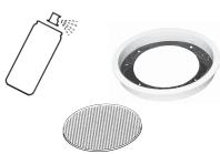
If desired, the speaker trim and grille can be painted to better match the installation environment. To paint trim remove the 4 socket head screws holding driver in place and disconnect the speaker. This will free the faceplate from the assembly.
