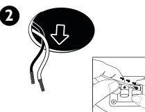
Strip wire and connect to the speaker terminals while ensuring that the polarity is correct.
