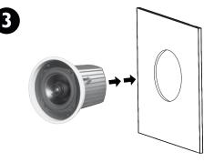
Before inserting the speaker into the cut material, ensure that the holding tabs are loosened and rotated to rest against the speaker assembly as seen in step 4. The grille must be removed to gain access to the holding tab screws.
