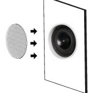
Insert press fit grille to complete the installation.
