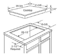
\*Depth of unit at conduit connection location (rear) is 6-1/4\* on models PP975/945 and 4-3/16\* on models CP350/850, PP944/962/932/912, and JP356/346. Depth of unit at baffle (front) is 4-5/8\* on models PHP960/900.
