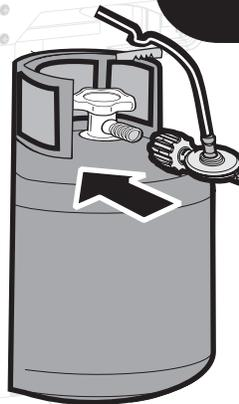
Tank must be secured and installed properly before you attach to Regulator.
