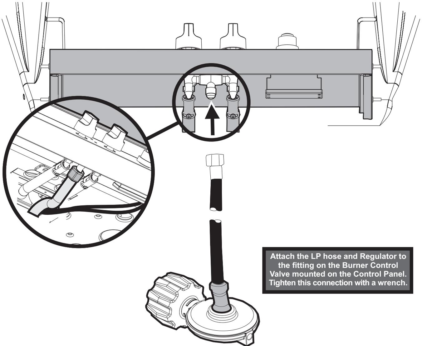
Attach the LP hose and Regulator to the fitting on the Burner Control Valve mounted on the Control Panel. Tighten this connection with a wrench.
