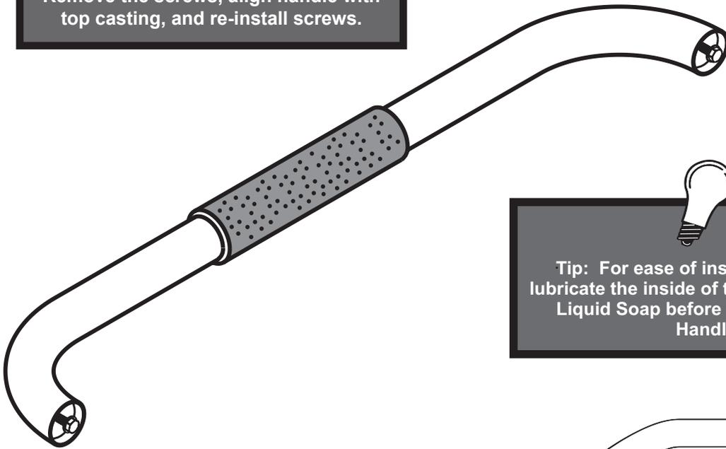
**Tip:** For ease of installation, lightly lubricate the inside of the Foam Grip with Liquid Soap before twisting it on to Handle.
