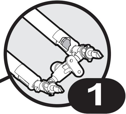
Slide the Venturi onto the Valve Assembly as shown.
