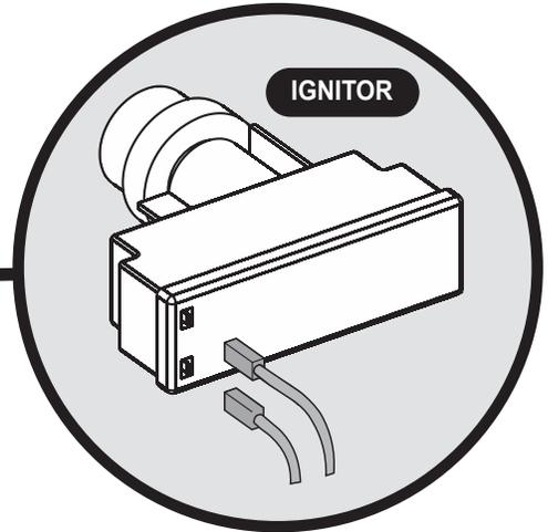
Route Leads from Collector Box and secure to Ignitor Terminals (polarity is not important).
