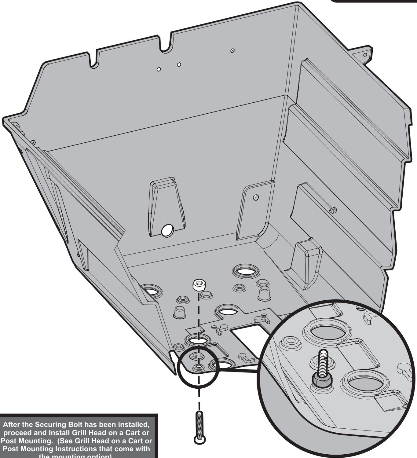
After the Securing Bolt has been installed, proceed and Install Grill Head on a Cart or Post Mounting. (See Grill Head on a Cart or Post Mounting Instructions that come with the mounting option).
