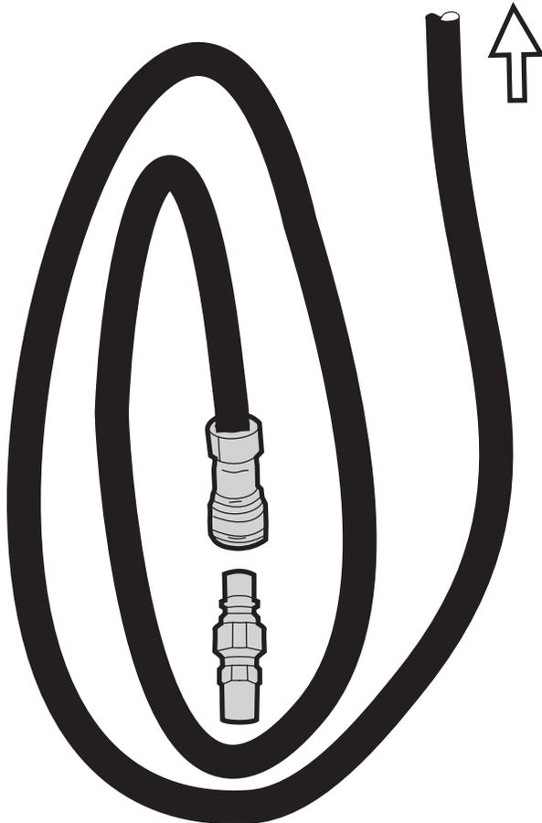
Attach the Natural Gas hose to the fitting on the Burner Control Valve mounted on the Control Panel. Snug this connection with a wrench.
