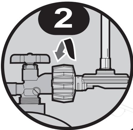
Inspect the threaded outlet on the tank and the threaded inlet on the grill's pressure regulator for dirt, nicks, or corrosion that might interfere with a gas-tight connection. If the tank outlet shows damage, return the tank to the supplier for a replacement. If the grill's pressure regulator shows nicks or other damage, contact your dealer for genuine Broilmaster replacement parts.
