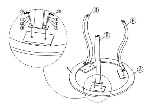
STEP 2: Place the Shelf (C) onto the bottom of the Table Leg (B) and secure it with Flat Washer (3), Lock Washer (2), Bolts (1) into the holes of the Table Leg (B) by using Allen Key (4) and fully tighten all Bolts (1).
