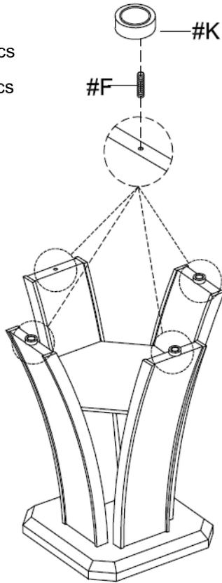
Insert the 4 threaded studs (#F) into the top of the stands (#3). Then insert the 4 spacers (#K) onto the 4 threaded studs (#F).
