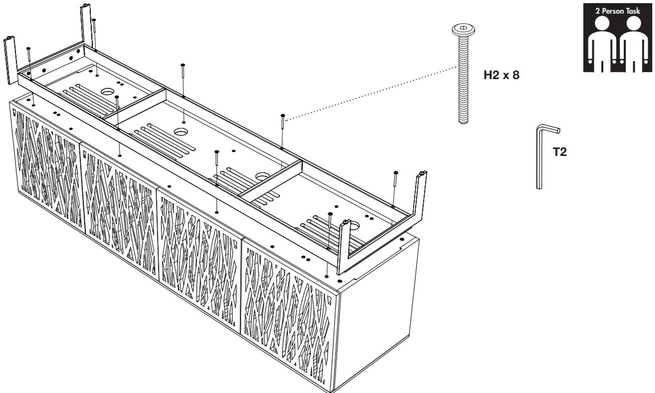
**Step 3 Triple** - With help from another person, carefully position the cabinet **A1** upside-down (as shown) or on its back. Attach the base to the cabinet with **8 Screws H2** using **Hex Wrench T2**. Do **NOT** fully tighten until all 8 screws are started.
