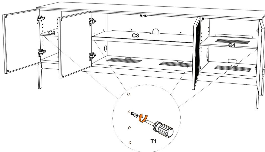
**Step 6** - The 2 **Back Panels C5** are removable and can slide towards the middle. To remove lift up and pull the bottom edge out of its groove. To re-install, put the top edge of the back panel into the top groove, then drop the bottom edge into the bottom groove.
