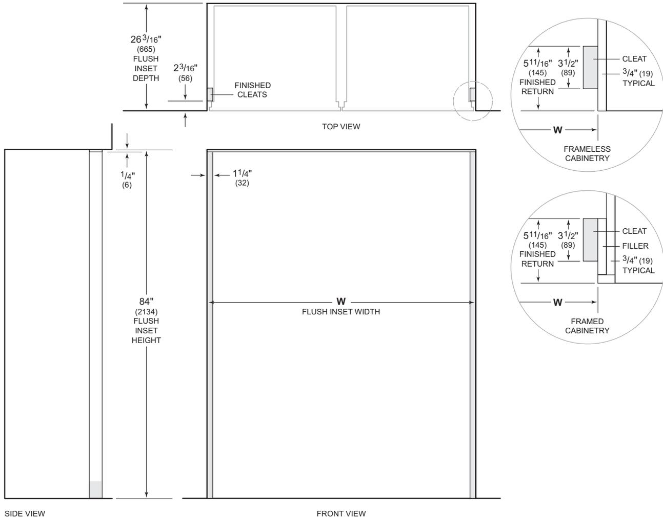
NOTE: 3 1/2" (89) finished returns and shaded areas will be visible and should be finished to match cabinetry. Shaded line represents profile of unit with 3/4" (19) panel.
