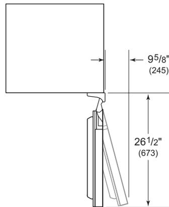
**IMPORTANT NOTE:** Overall dimensions do not include panels or handles. Dimensions will vary with panel thickness.
