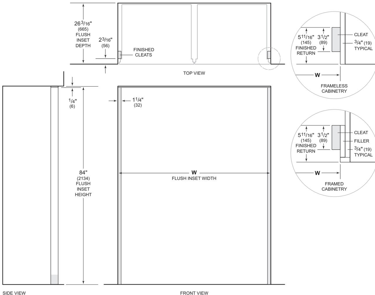
NOTE:  $3\frac{1}{2}$ " (89) finished returns and shaded areas will be visible and should be finished to match cabinetry. Shaded line represents profile of unit with  $3/4$ " (19) panel.
