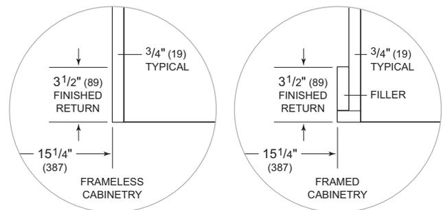
The depth of the unit is 23" (584). Allow for panel thickness when planning the finished opening depth. A minimum 3 1/2" (89) finished return is required on all sides of the opening. Framed cabinets require additional finished filler material behind the face frame for a proper installation. Refer to the illustration above.
