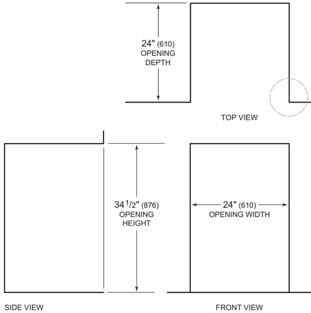
The depth of each model is 23 1/8" (587). Allow for panel thickness when planning the finished opening depth. A minimum 3 1/2" (89) finished return is required on all sides of the opening. Framed cabinets require additional finished filler material behind the face frame for a proper installation. Refer to the illustration.
