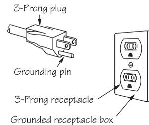
**⚠ WARNING** Improper use of the grounding plug can result in a risk of electric shock. **Do not use an extension cord. If the power supply cord is too short, have a qualified electrician or serviceworker install an outlet near the appliance.**
