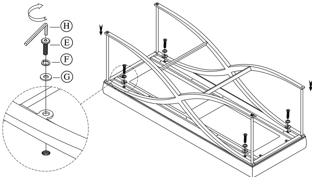
STEP 4: Re - attach metall frame all the screws from step 1
