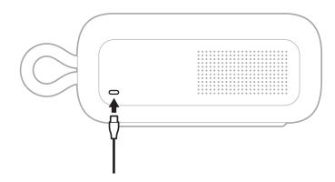
2. Connect the other end of the USB-C cable to a power source such as a computer or wall charger.
