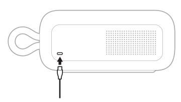
2. Connect the other end of the cable to the USB-C port on your device.
