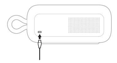
2. Connect the other end of the USB-C cable to a USB-C power supply.
