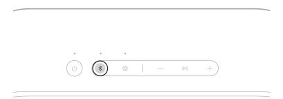
2. Within 2 seconds, press the *Bluetooth* button *∛* again to hear the name of the next device in the speaker device list.
