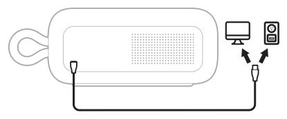
While charging, the battery light pulses white. When the battery is fully charged, the battery light glows solid white.
