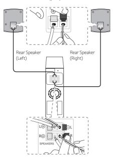
2. Connect the wireless receiver and the rear speakers (right, left) with the speaker cables.
