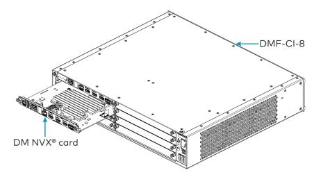
3. Finger-tighten the two captive panel screws to secure the card—do not overtighten the screws.
