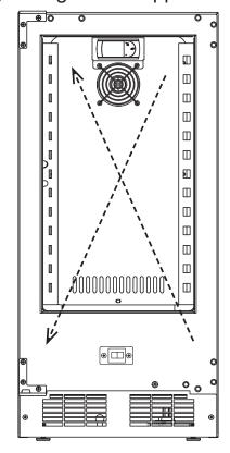
**Step 10**. Rotate the door 180° and attach it to the cabinet using the SC-541-SS upper screw and the SC-542-SS lower screw. See figure 12.
