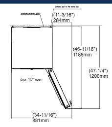
Allow door swing clearance at locations next to a wall. If the appliance is installed with the hinges next to a wall, the distance between the appliance and the wall must be at least  $1\frac{1}{2}$ " (40 mm). This is how far the handle protrudes when the door is open.
