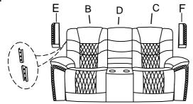
STEP 2:Install the LSF backrest (B), Console back (D), and RSF backrest (C) by align and insert the metal bracket to the metal brackets of the seat (A).Please make sure the brackets and console back are inserted all the way and secured into position.
