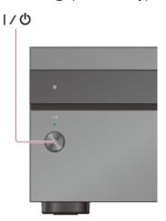
You can also turn on the receiver using MAIN I/(1) (on/standby) on the remote control. To turn off the receiver, press MAIN I/(1) (on/standby) again.
