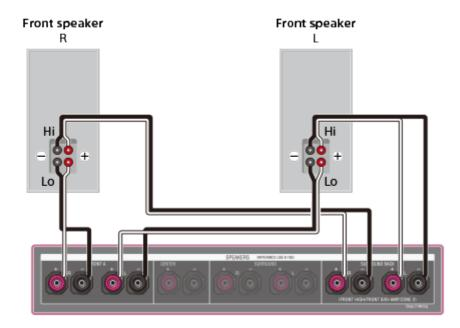
Connect the jacks on the Lo (or Hi) side of the front speakers to the SPEAKERS FRONT A terminals, and connect the jacks on the Hi (or Lo) side of the front speakers to the SPEAKERS SURROUND BACK/FRONT HIGH/FRONT B/BI-AMP/ZONE 2 terminals. Make sure that metal fittings of Hi/Lo attached to the speakers have been removed from the speakers to avoid receiver malfunction.
