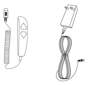
Attach the control wand pin plug to the matching pin plug at the rear of the seat. Make sure to lock the 2 pin plugs together using the snap lock. Follow the routing of the control wand wiring as seen beside.
