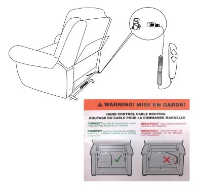
Attach the lead wire from the power motor found attached at the rear of the lift chair to the power adapter.
