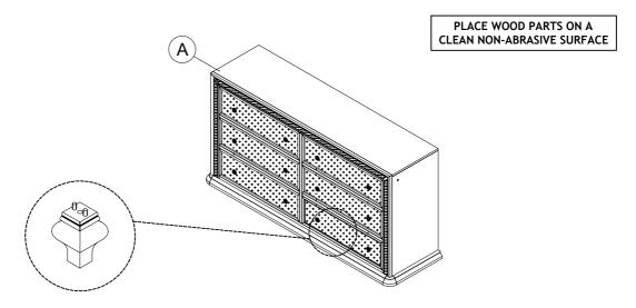
**STEP 2**: Install the LEG (B) by using the ALLEN KEY (3) with hardware
