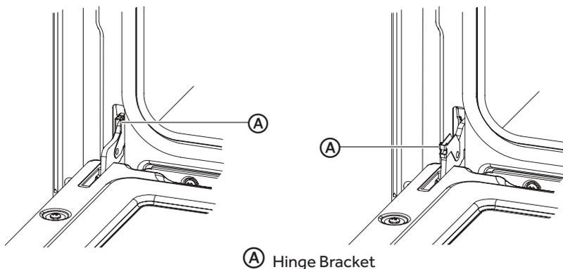
3. Holding the door firmly, close the oven door completely.
