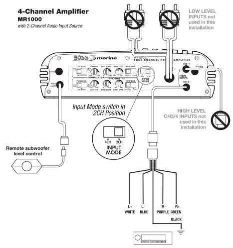
To LEFT and RIGHT Speaker Terminals of head unit or signal processor
