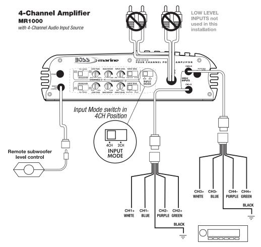
To FRONT and REAR L/R Speaker Terminals of head unit or signal processor
