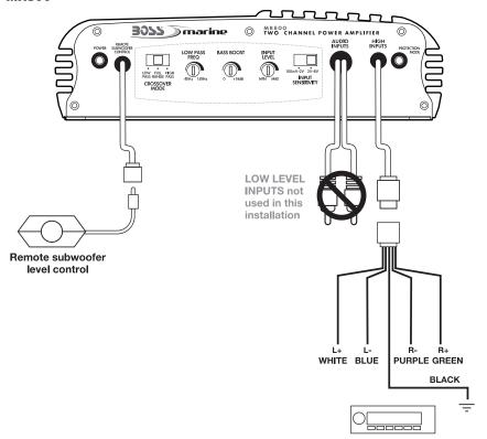
To LEFT and RIGHT Speaker Terminals of head unit or signal processor
