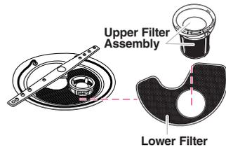
**IMPORTANT:** To avoid damage to dishwasher, do not operate your dishwasher without filters properly installed. Be sure lower filter is securely in place and upper filter assembly is locked into place. If upper assembly turns freely, it is not locked into place.
