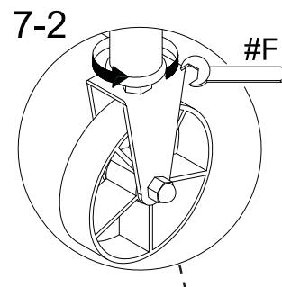
2. Turn right to tighten the wheel using the wrench (#F).
