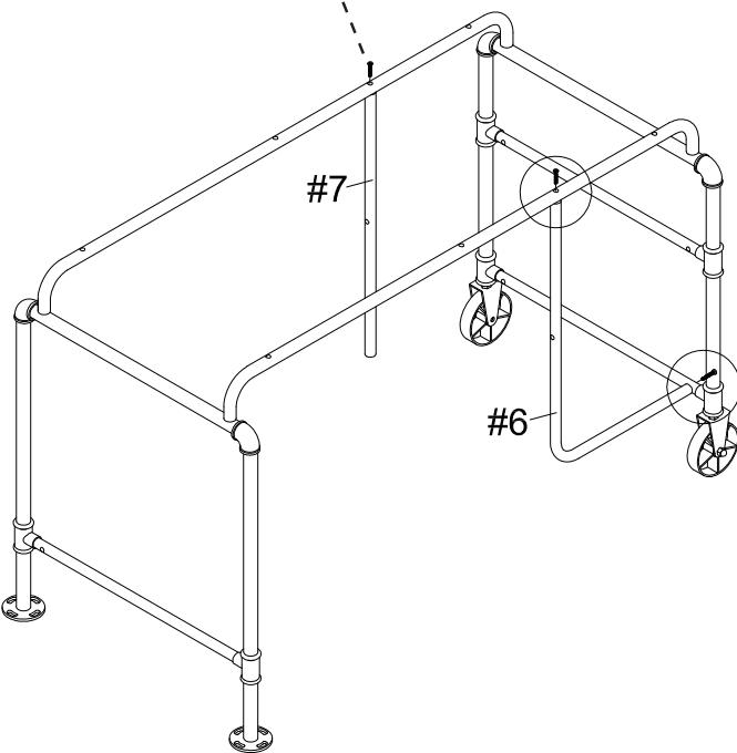
1. Align the long end of the front shelf post (#6) to the hole along the top support tube (#4), then insert a bolt (#D) and secure.
