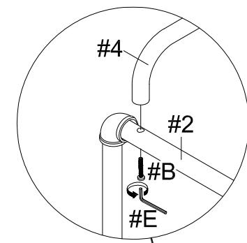
Align the top support tubes (#4) to the holes along the top of the right and left side panels (#2,3), then insert the bolts (#B) from below. Secure using the Allen wrench (#E).
