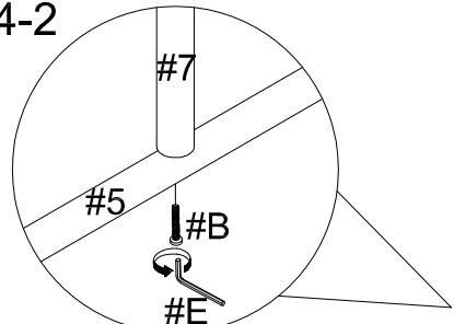
1. Align the rear connect tube (#5) to the holes along the bottom sides of the left and right side panels (#2,3), then insert a bolt (#B) into each end. Secure using the Allen wrench (#E).
