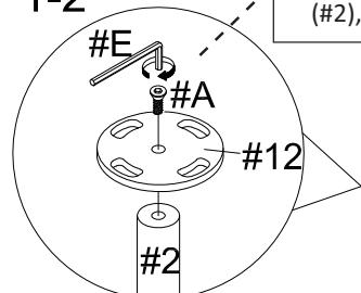
2. Place the leg plates (#12) onto the left side panel (#2), then insert a bolt (#A) into the center, secure.
