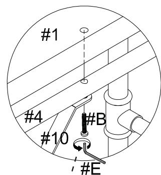
Place the desk top (#1) on top and align the holes. Insert a total of 6 bolts (#B) from below and secure using the Allen wrench (#E).
