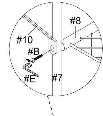
Align the upper shelf (#8) to the holes along the sides of the posts and panel. Insert a bolt (#B) into each hole and secure using the Allen wrench (#E).
