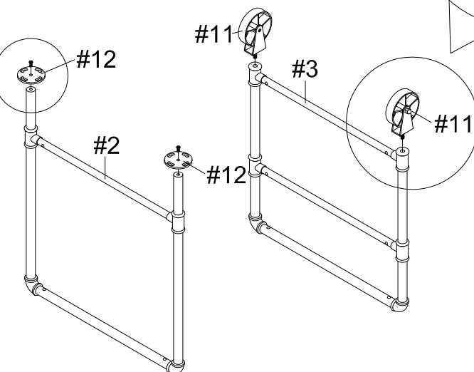
1. Insert the threaded ends of the wheels (#11) into the holes along the bottom of the right side panel (#3). Turn right to tighten.
