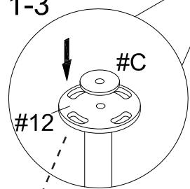
3. Place a floor protector onto the leg plates (#12).
