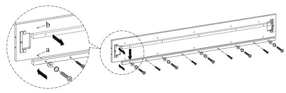
STEP 5: Screw the bolts(H) into HB & FB. Make sure the slat bearer is in the position (a). Align the bolts with the holes in the end of side rails and attach the side rails to HB & FB using Flat Washer (I), lock washers(J) and nuts (K). Then use a hex wrench to tighten all the nuts.
