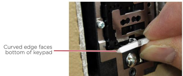
Figure 4. Sensor bar with split up/down buttons
