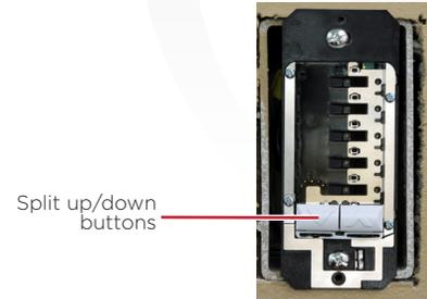
Orient the button assembly so that the up button is on the right, and then slide the mounting holes at the bottom of the button assembly over the small black prongs that stick out at the bottom of the keypad button area.
